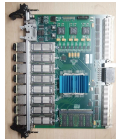
5 SSP Fiber-Optic DAQ (compatible with CLAS12)
