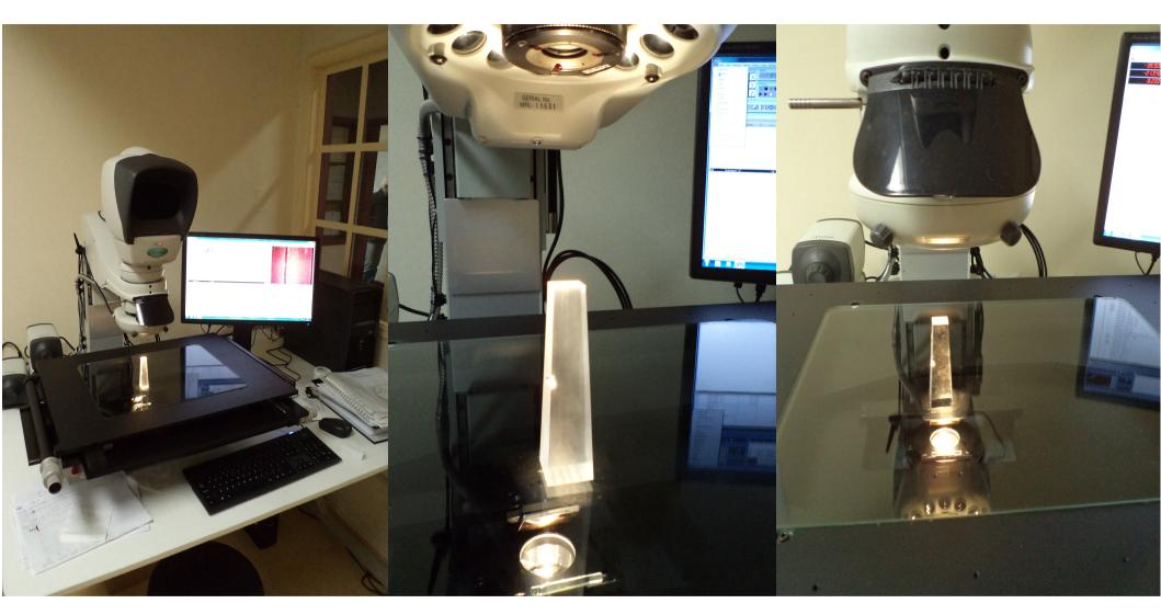
Vision engineering Hawk 5000 monodynascope Provides measurements with 3mk accuracy While light guides can have ~127mk tolegance
