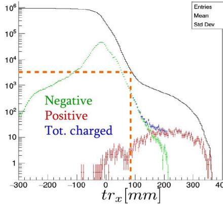
Total charged particle rate at  $x > 90$  mm is less than 4KHz
