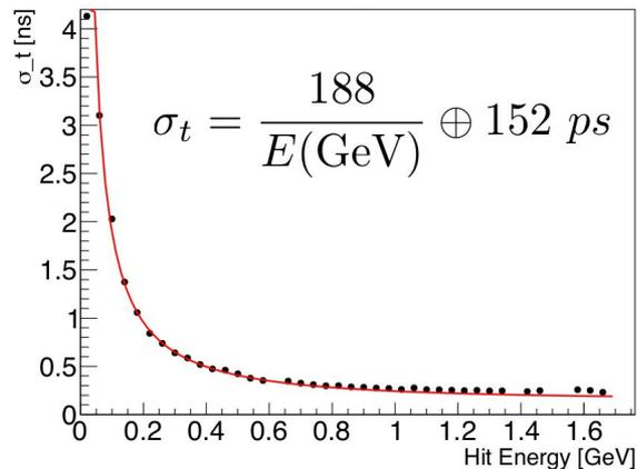
Good time resolution allows for ps Cluster coincident time resolution  $\rightarrow$  used to identify  $e^+e^-$  pairs with high accuracy
