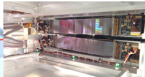
Six layers of pairs of Si microstrip sensors → One axial and the other at small angle stereo (50 & 100)
