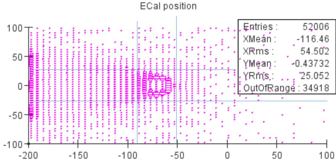
It looks like electrons passing through the ECal hole are creating low-E hits/clusters, while being assigned tracks
