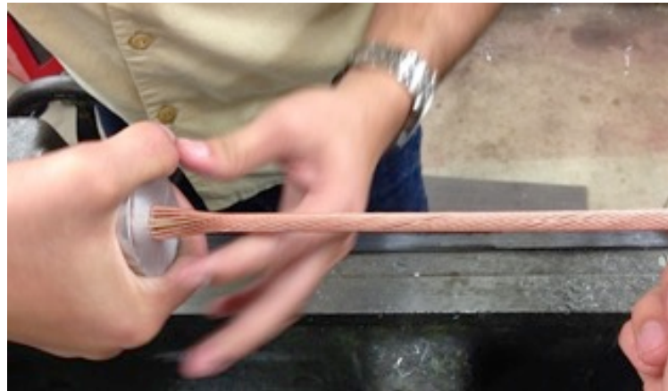
15 NbTi/Cu wires are cabled onto a perforated spring tube.
