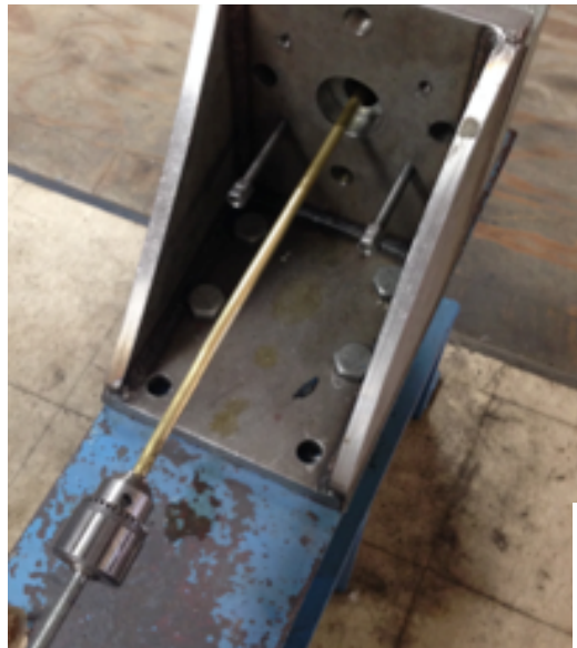
The cable is inserted in a sheath tube, and the sheath is drawn onto the cable to just compress the wires against the center tube.
