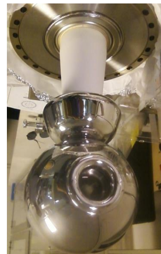
First insulator conditioned to 325 kV
