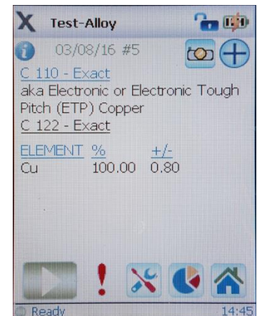
Non-destructive characterization using XRF (x-ray fluorescence spectroscopy)
