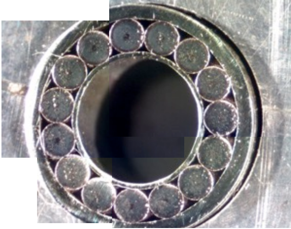
The cable is inserted in a sheath tube, and the sheath is drawn onto the cable to just compress the wires against the center tube.
