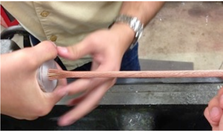
Superconducting wires are cabled onto a perforated center tube.
