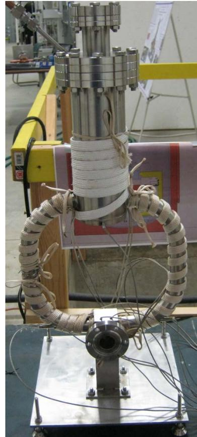
Density differential between hot and cold leg drives flow
