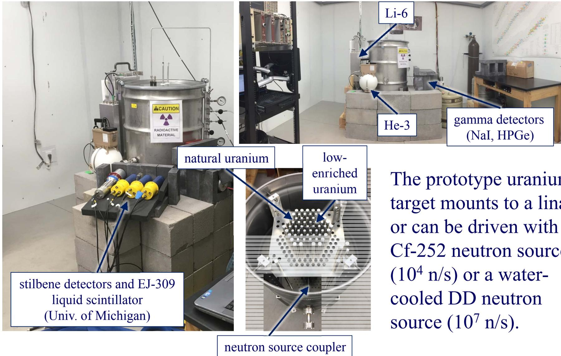
The prototype uranium target mounts to a linac or can be driven with a Cf-252 neutron source ( $10^4$  n/s) or a water-cooled DD neutron source ( $10^7$  n/s).
