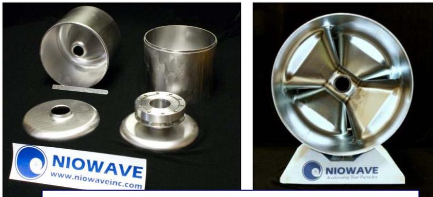
Superconducting niobium cavities
