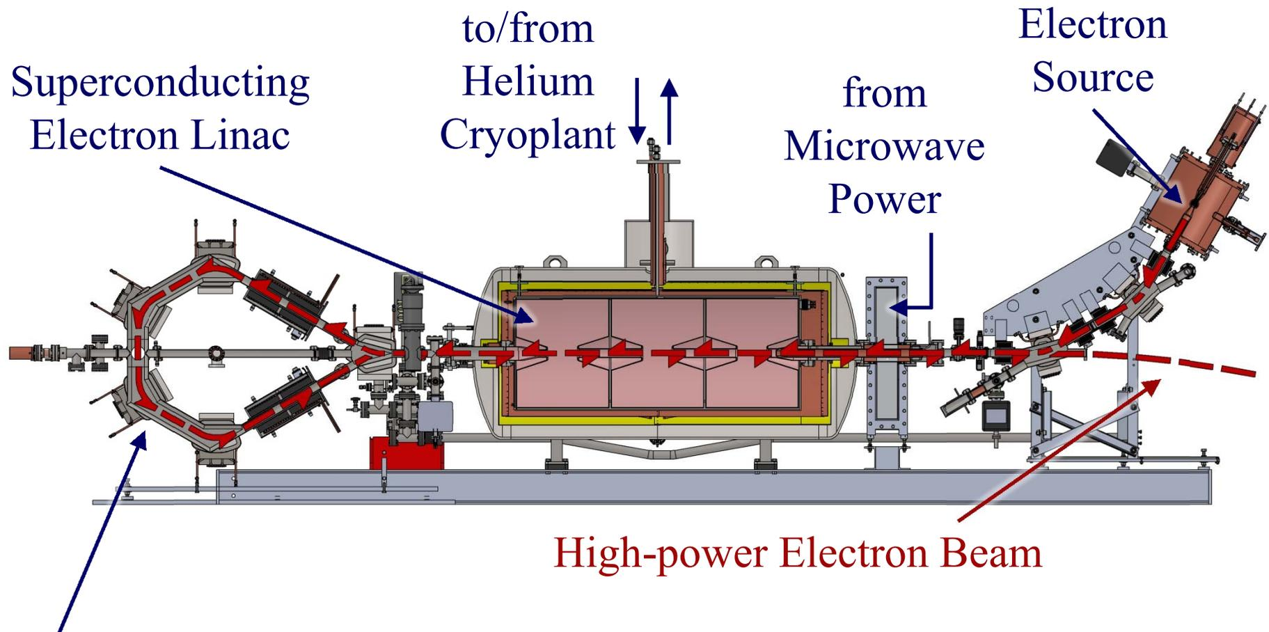
In this design, a magnetic arc (at left) brings the beam through the accelerator a second time, reducing costs for the cryomodule and refrigerator.
