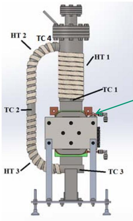
Verified flow with 200 A current through lead-bismuth eutectic
