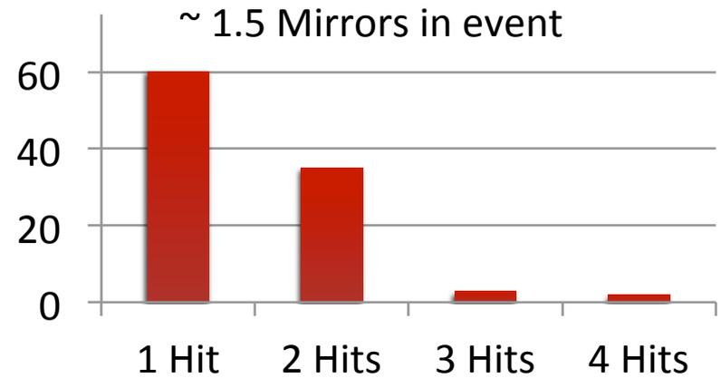
Cerenkov radiation from single electron may split between mirrors and is collected by different PMTs
