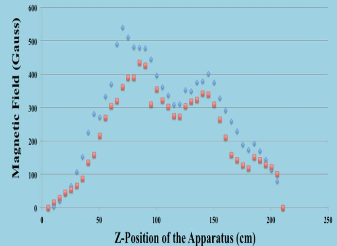
X-Component of the TORUS Field with Tube C in Hole C
