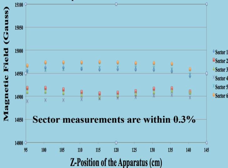
Y-Component of the TORUS Field at Hole B
