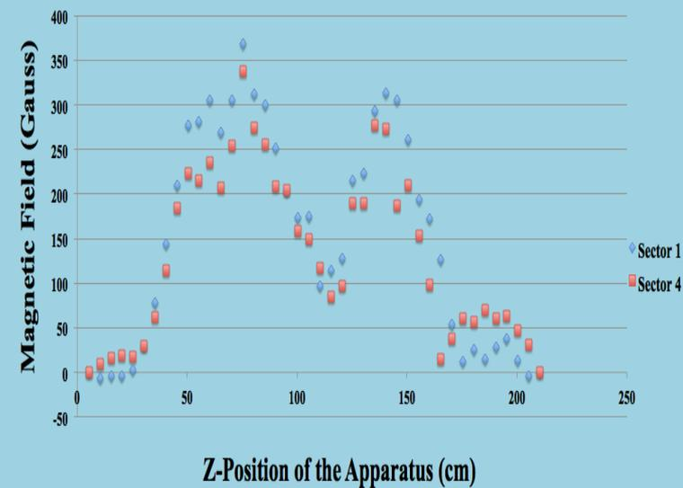
Fig. 12. X-component of the TORUS field at Hole C using different non-magnetic tubes to test for non-field effects to data
