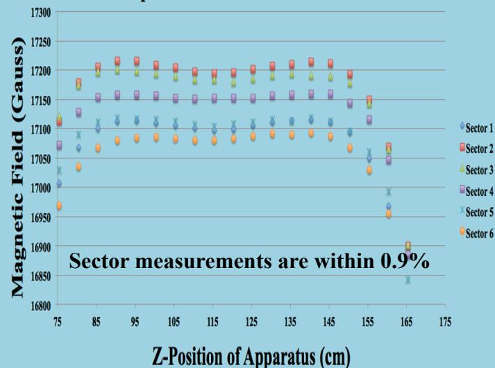
Y-Component of the TORUS Field at Hole C
