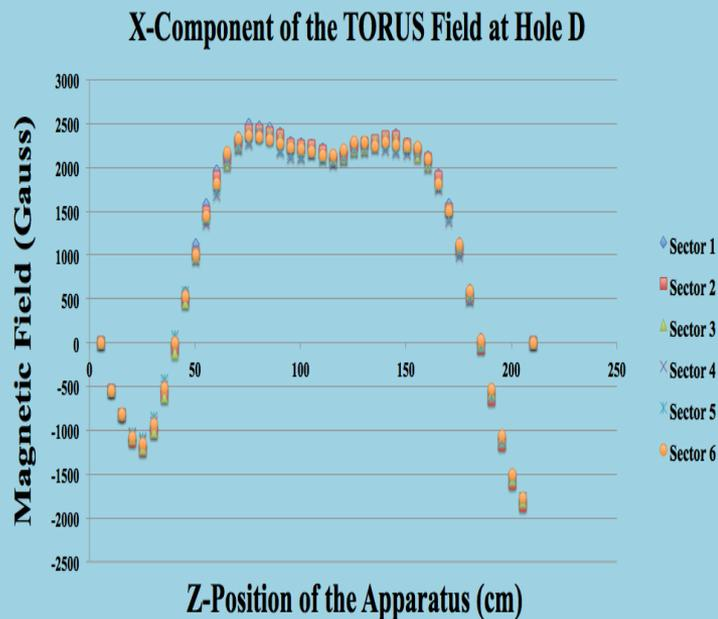
Fig. 11. X-component of the TORUS field at Holes A-D in Sectors 1-6.
