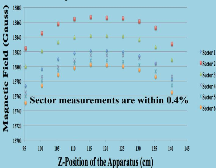
Y-Component of the TORUS Field at Hole D
