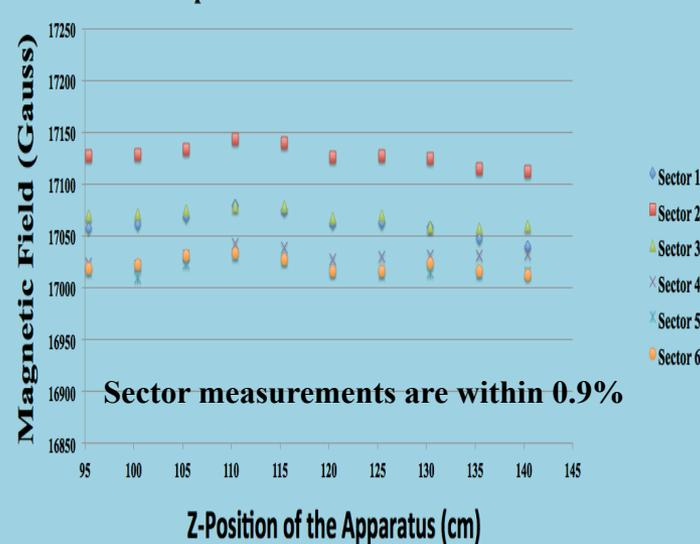
The y-component, which points in azimuth, was measured with great precision
