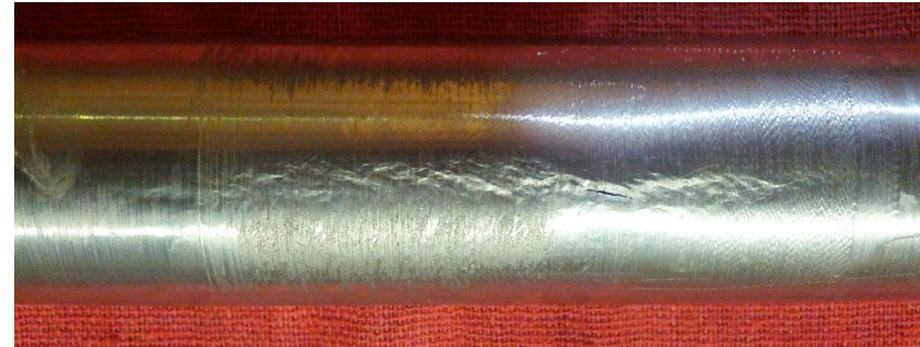
As expected, failed at weld
