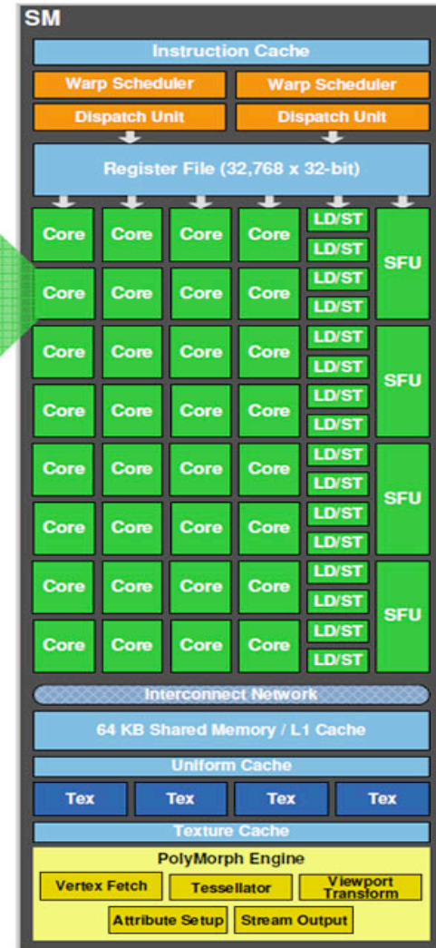
Streaming Multiprocessor (SM)
