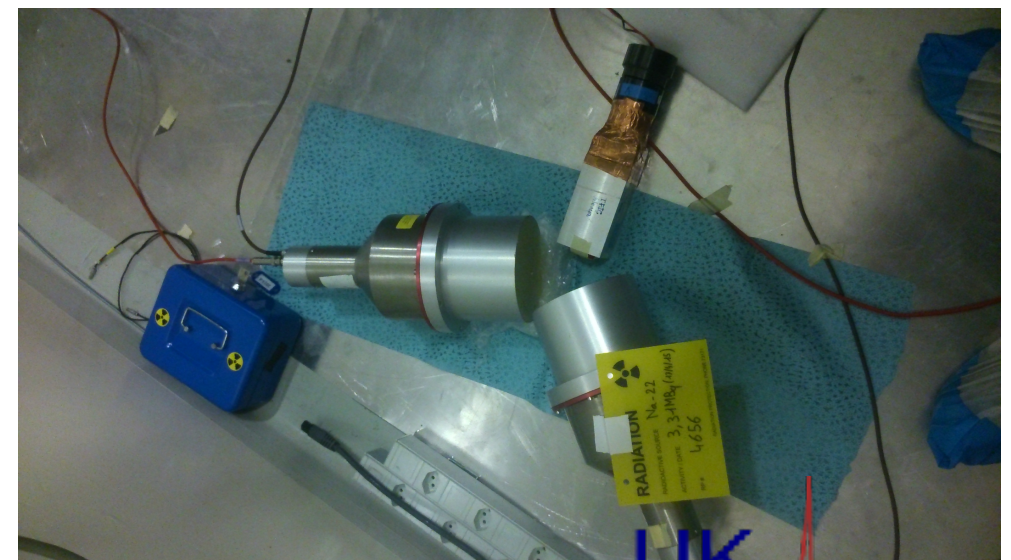
Calibration of two Nal and one LaBr 3 detectors
