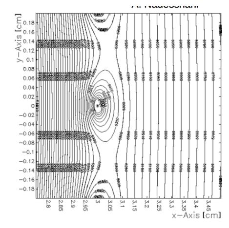
Cover end plates with a resistive paint to have a homogeneous electric field
