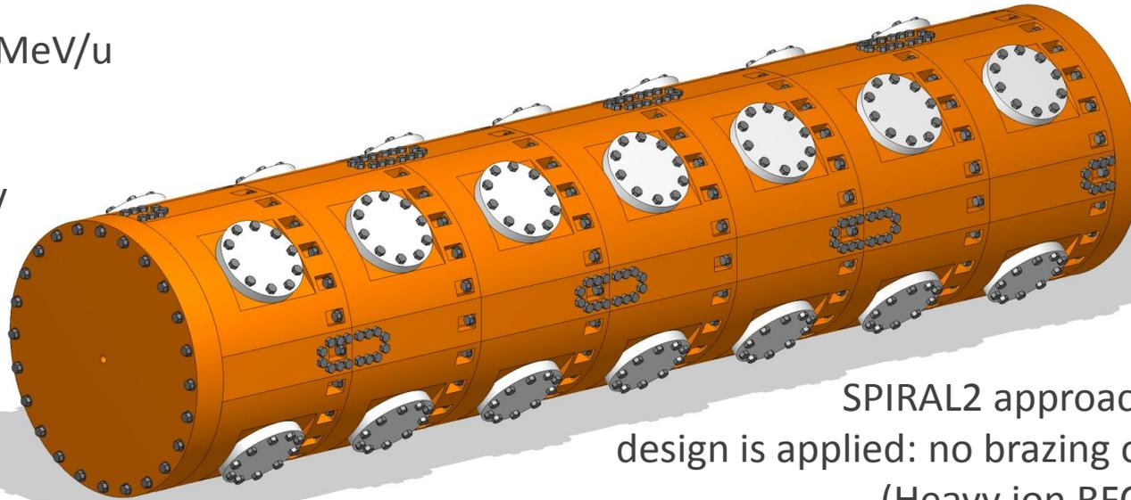
SPIRAL2 approach to mechanical design is applied: no brazing or welding joints
