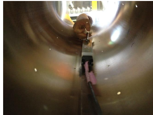
Measure inside magnetic shield by using 3-axis flux gate sensor.
