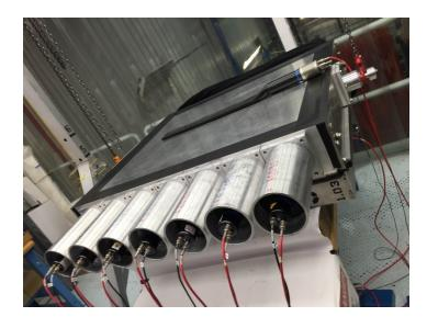
Good performance with cosmic ray tests with tray of n=1.03 Aerogel with "wrong way" muons.
