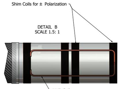
(Shown is a single NMR coil pair for a single target, although there will need to be 2 separate NMR circuits for the two targets  $\pm$  polarized)
