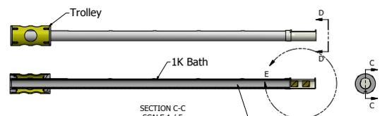
Re-entrant Beam Line (Low Pressure 1K gas, same volume as Pump Space)
