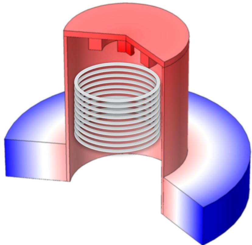
All ambient field is trapped up to a threshold field above which field can be expelled
