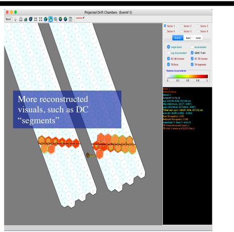
New "Projected Drift Chambers" view. Instead of the entire detector projected onto a constant  $\phi$  plane, each superlayer is projected onto a plane perpendicular to its wires. This reduces distortion and makes visualization of tracks and segments wrt DOCAs more accurate and, consequently, more useful.
