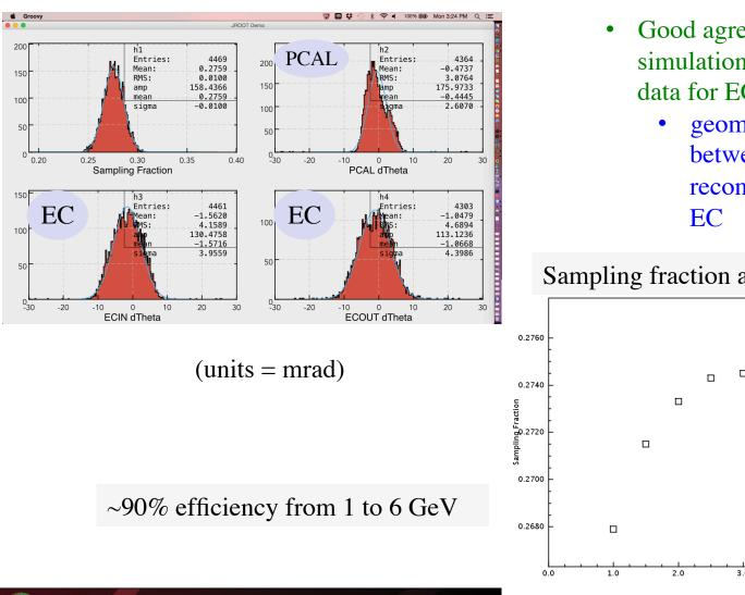
6 GeV photon simulated with GEMC
