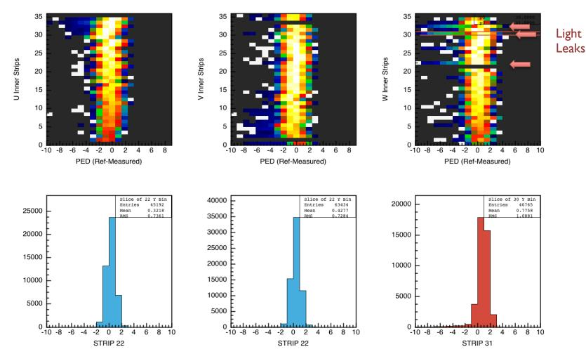
FADC Mode 7 provides event-by-event pedestals. Used to monitor luminosity related noise levels, light leaks, etc. by comparing to reference pedestals measured under normal conditions.
