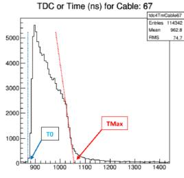
Knowledge of TMax can be useful in monitoring the DC condition and performance. For example, if the gas density changes, TMax will change.
