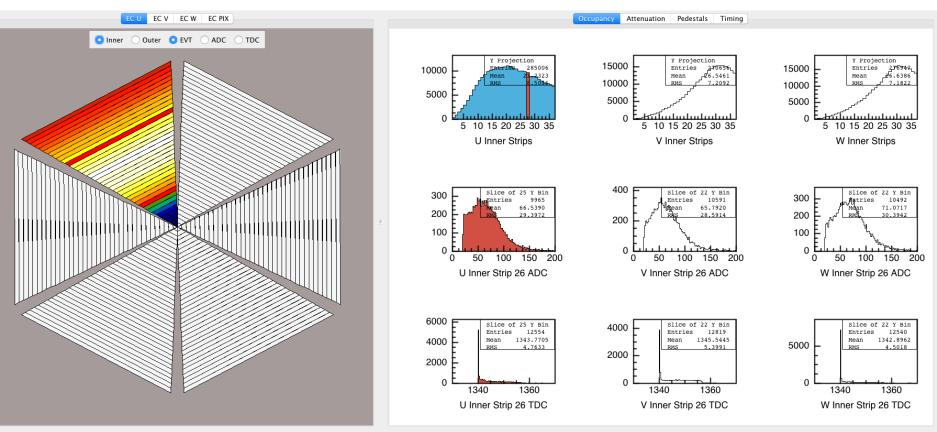
Detector panel (left) allows navigation at the strip level (ECU, ECV, ECW) or pixel level (EC PIX). Detector elements color-coded with events (EVT) or mean ADC, TDC values.
