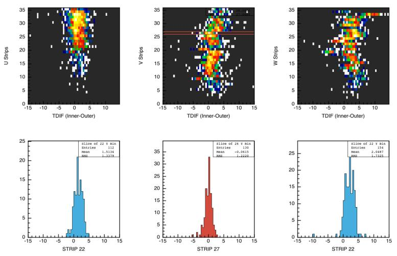
Time difference between EC Inner, Outer strips can be used to monitor quality of time calibration, changes in offsets, noise, etc. FADC Mode 7 timing shown here.
