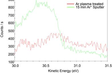
The reduction of oxygen and carbon produced a sharp Fermi edge from which a work function value of 4.27 eV was determined.
