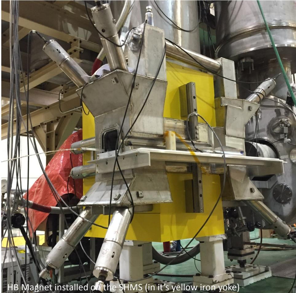
HB Magnet installed on the SHMS (in it's yellow iron yoke)
