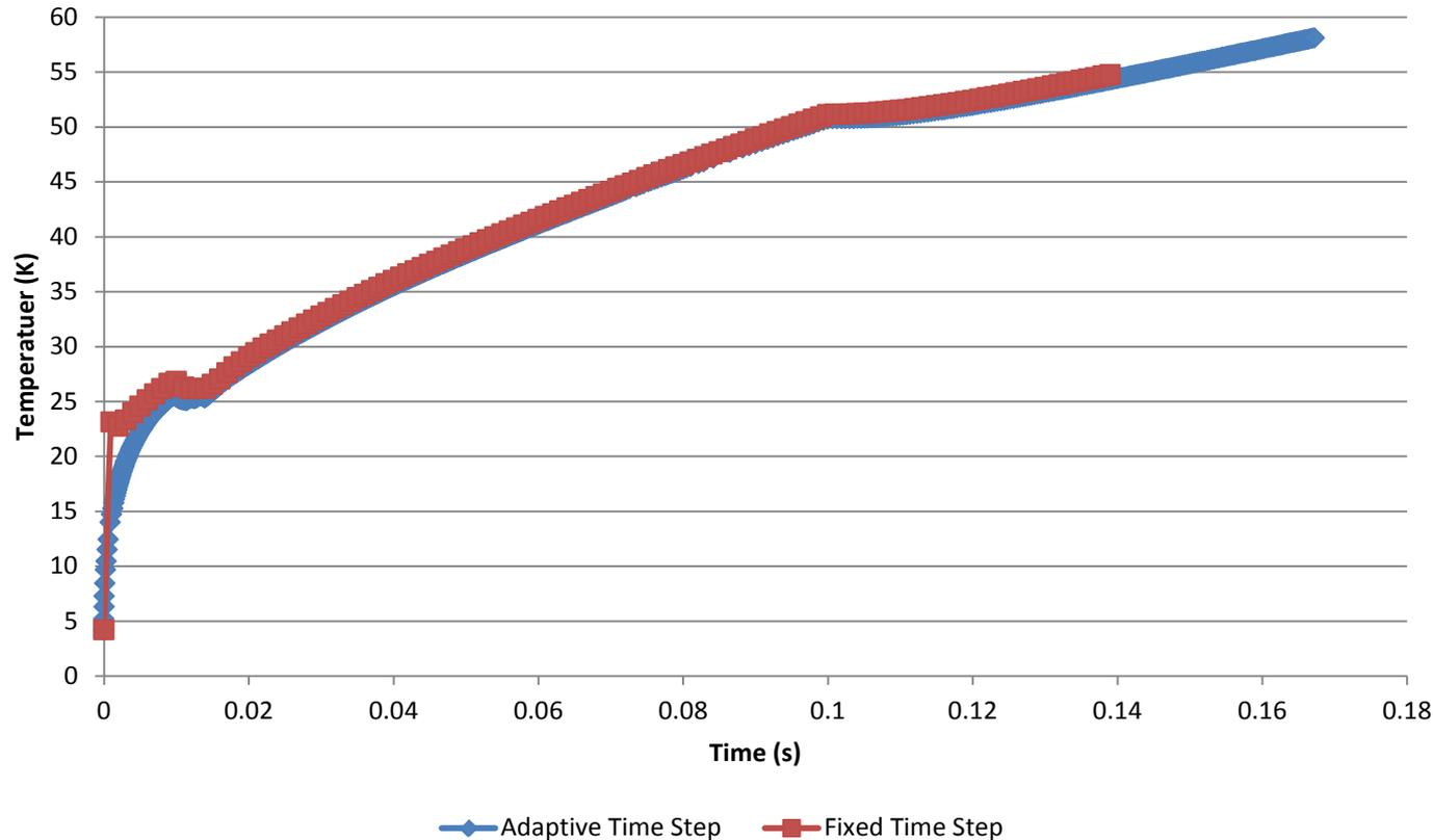
This is from one of the initial analysis at 3930 A, without time delay. This shows, that the simple time step is adequate for these quench calculations
