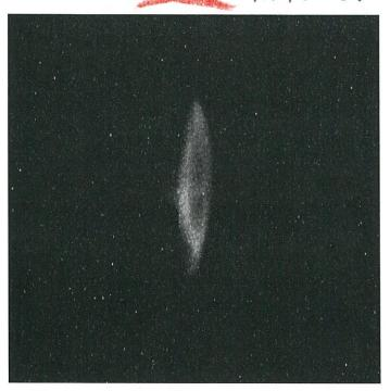
ITV0F06. The beam should be in the center of the viewer. This can be easily determined if the viewer lamps are turned on.
