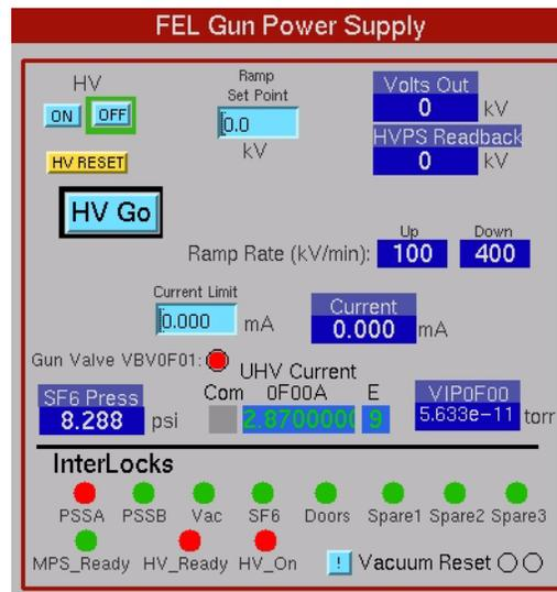
Figure 4-1: FEL Gun Power Supply Screen
