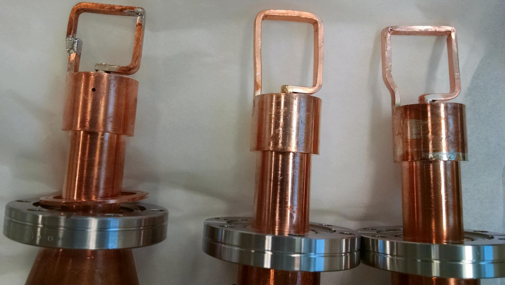
Modified coupler geometries being compared
