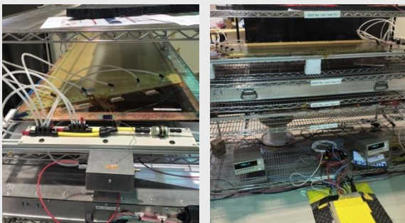
2nd prototype with gas manifolds (left); cosmic stand with hodoscope and picoammeters (right)
