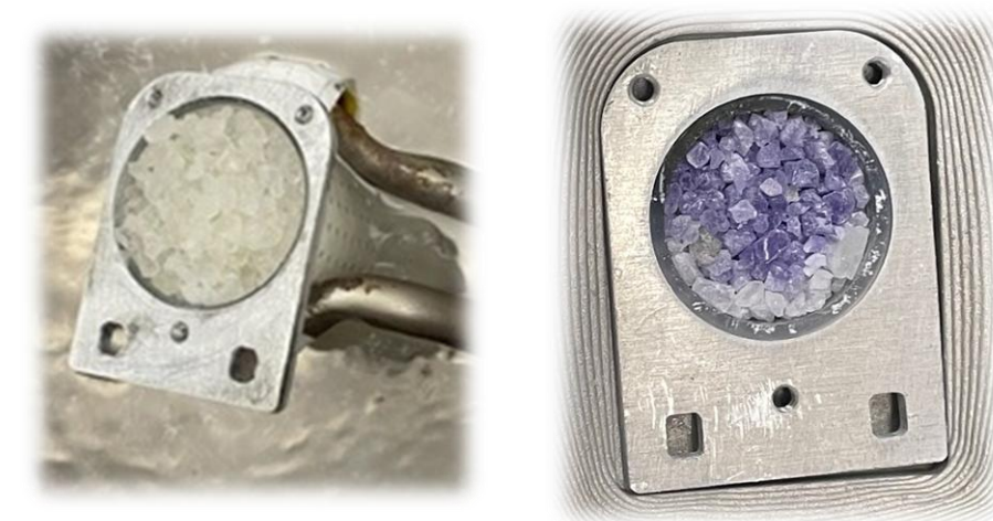
Ammonia crystals unexposed to beam (left), crystals after beam exposure (right). Purple color from paramagnetic centers.
