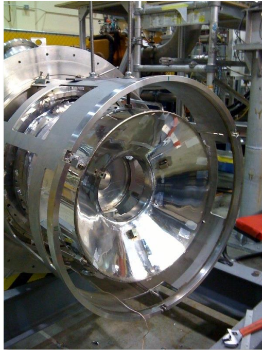
Vacuum can and heat shield removed
