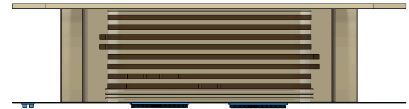
a side view perspective of the readout, 3 GEM layers, 8 layer field cage, cathode layer and the spacers between the layers.
