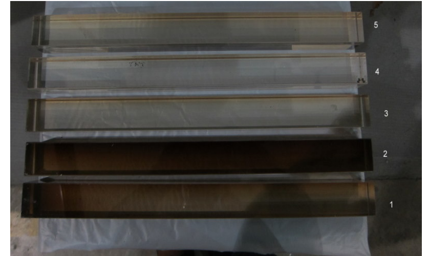
Figure 6 The lead glass blocks used to monitor the radiation dose after the C16 was placed at 10^\circ and there was 20uA beam on the 15cm LH2 target. Block 1 was placed parallel to the C16 along the beamline side of the C16. Block 1 has damage at the front (left side of photo) and along the side. Block 2 was placed in front of the C16 and perpendicular to the front face. Blocks 3,4 and 5 were located at different locations on the spectrometer platform that was near 30^\circ . These blocks show only moderate damage.
