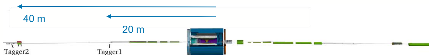
Figure 7: ePIC Low- Q^2 Tagger in Far Backward region.
