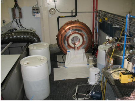
FIGURE 8. Setup of Electropolishing for the 201 MHz cavity.
