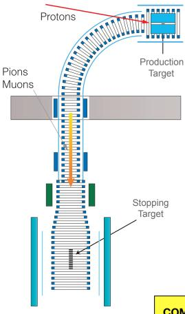
Intense Pulsed Proton Beam 8GeV-3.2kW (12 days)
