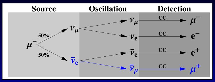
This requires a detector which can distinguish  $\mu^+$  from  $\mu^- \Rightarrow$  magnetic field of around 1T
