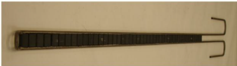
The first Titanium-tube water cooling line prototype
