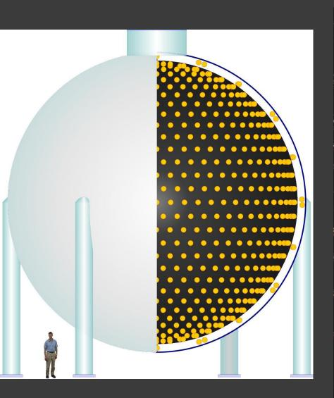
541 meters downstream 3 meter overburden •12 meter diameter sphere (10 meter "fiducial" volu Filled with 800 t of pure mineral oil (CH) (Fiducial volume: 450 t 1280 inner phototubes, 240 veto phototubes
